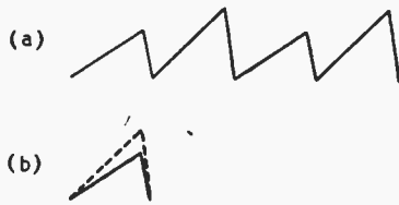
Fig. 2. Alternate saw-teeth are of different amplitude here (a); this is more easily seen in (b) where two cycles are superimposed.
