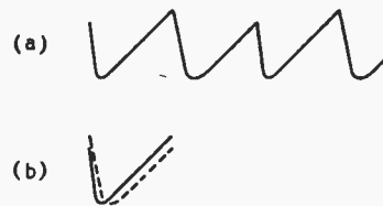
Fig. 3. Regularly recurring waves of different fly-back time are illustrated at (a). Two cycles are superimposed (b).
