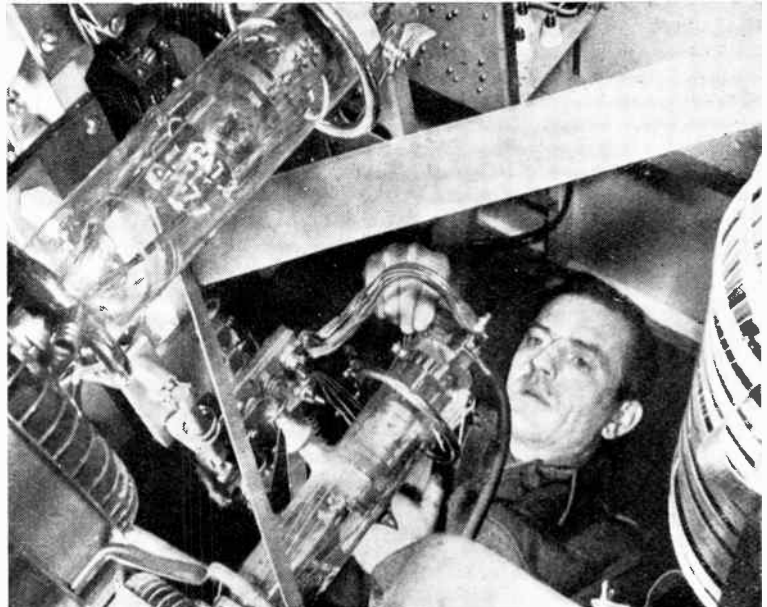
Royal Canadian Air Force photograph The filament leads being replaced on an air-cooled CAT3 valve on arrival at a new site
