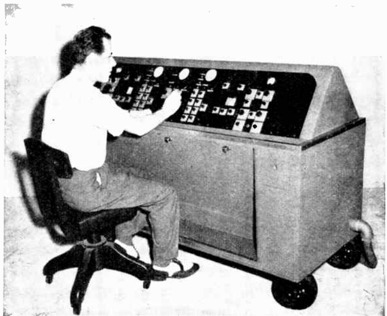
THE TELEMOBILE portable control desk for use with two television cameras. The equipment is mounted on hinged chassis which can be opened out for maintenance. It operates from AC and several units can be employed together if more than two cameras are used. It is designed by Television Products Inc., Hollywood, U.S.A.
