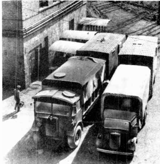
MCN parked in a factory yard in Germany. The transmitter trailers are in the rear while the studio and stores vehicles are in the foreground. In this instance factory chimneys were used for supporting the aerial.
