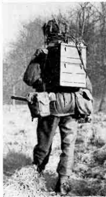
FM "WALKIE-TALKIE." This American Signal Corps pack transmitter-receiver, type SCR 300, has been used to some extent by the British Army. The set, measuring 17" x 12" x 7 in., weighs 35 lb.
