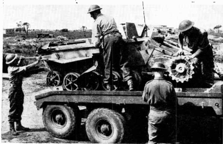
THE FIRST of the much-talked-of German radio-controlled "tanks" to fall into our hands. Having driven the vehicle, carrying an 800 lb. explosive charge, towards its objective the driver dismounts and directs it by radio for the final few hundred yards. It then drops its charge, which is fitted with a time fuse, and is backed to the driver by radio control. The vehicle, 12 ft. long, 6 ft. wide and 4 ft. high, is slightly smaller than a Bren carrier.
