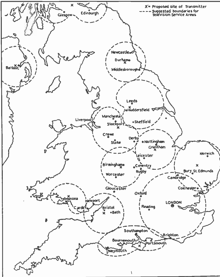
Map showing proposed location of stations for providing a television service for the more densely populated areas of the country. Each television zone would also be served by a group of FM sound broadcasting stations.
