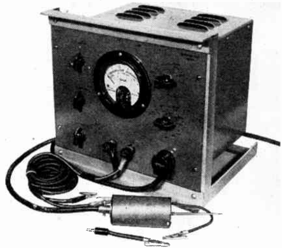
Front view of test meter showing range switches and zero setting controls.
