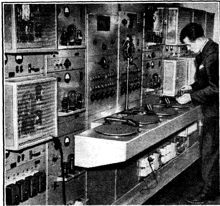
FROM THE BROADCASTING ROOM in the Tower of Empire at the Empire Exhibition, Glasgow, have been radiated on an average sixty SOS messages a day, apart from the ordinary programme, during the six months' run of the exhibition, which closes on October 31st. Equipped by the General Electric Company, the system involves 15 microphone points and 130 loud speakers in various parts of the grounds.
