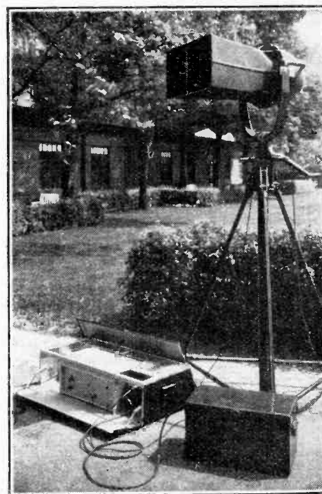
PORTABLE PA. Intelligible speech can be heard up to 600 feet on a 20-degree beam with this new Telefunken outfit. The amplifier output is rated at 20 watts.
