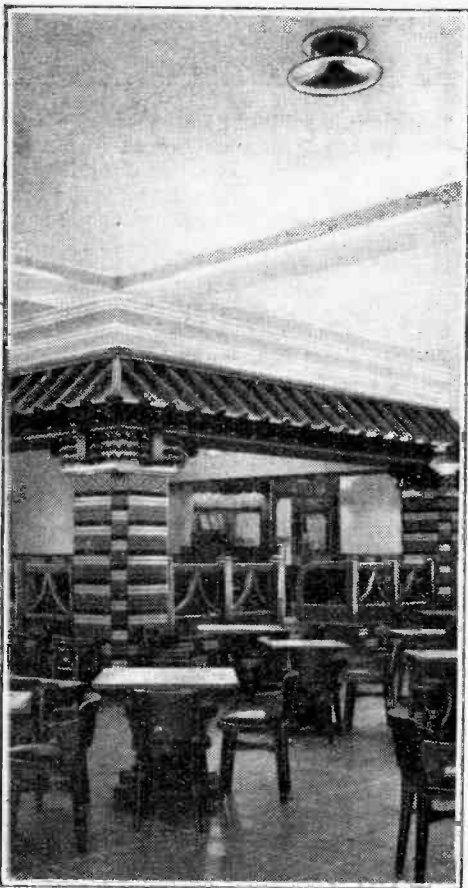
In the Brasserie at the Coventry Street Corner House. One of the ceiling speakers with a deflector to facilitate the downward diffusion of sound is seen.
