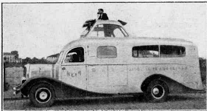
A VANTAGE POINT is secured for French commentators when using this reporting car. As can be seen, the roof of the observation cabin is hinged allowing an uninterrupted view for the commentator.
