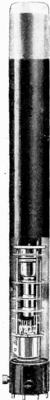
Fig. 4.—Cossor 2-in. tubular high-vacuum cathode-ray tube.
