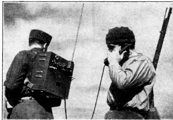
TWO-WAY COMMUNICATION is being maintained during the Spanish war by the use of ultra-short-wave transmitter-receivers. As can be seen from this picture the complete apparatus is easily carried on the back of an infantryman.
