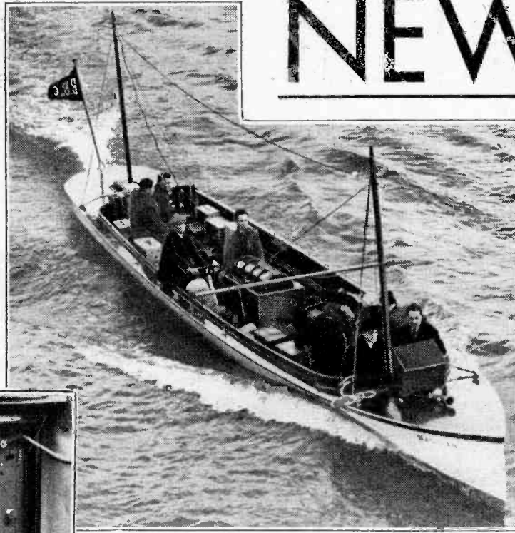
THE B.B.C. LAUNCH Magician , which is used for boat-race commentaries and descriptive broadcasts from the Thames, is equipped with a 100-watt Marconi transmitter (inset) designed to work on the 40-120 metre waveband. The engineers experiment until they find the frequency best suited to the local conditions and the transmissions are picked up by a receiving station located near-by.
