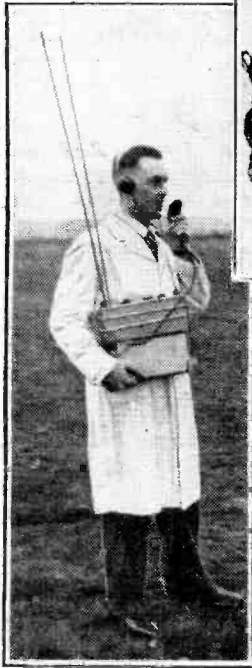
RADIO-TELEPHONE equipment developed in Germany for use in gliders and sail-planes. The complete equipment, which weighs only 9¼ lb., and measures but 12in. overall, is shown above with phones and midjet microphone. On the left, it is being used as a ground station.
