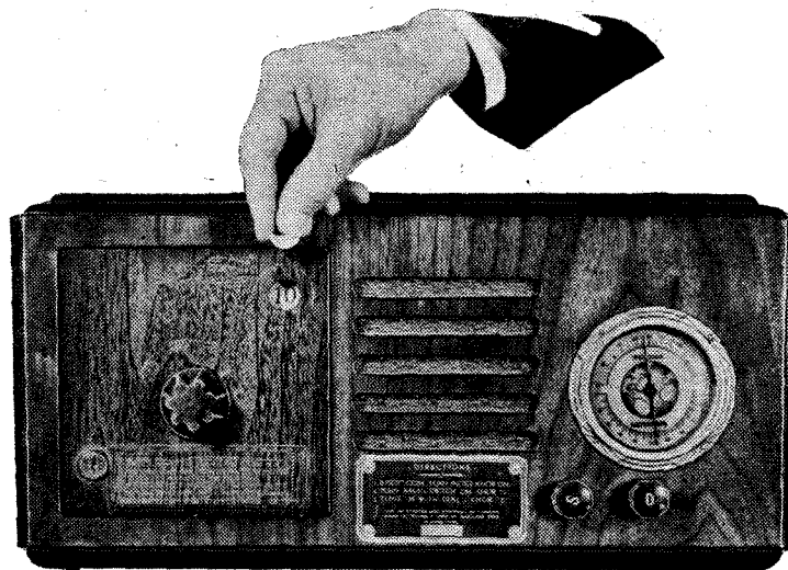
PAY WHILE YOU LISTEN. An automatic 5-valve superhet receiver of the type being installed in hotels in America. The insertion of a coin enables the set to be operated for either half an hour or an hour. A wide range of home and foreign stations can be tuned in.
