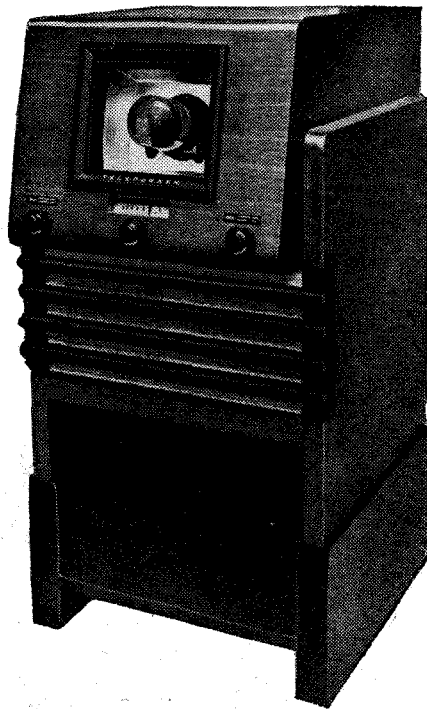
A television receiver designed for the projection of pictures. It is made by Telefunken.
