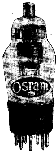
The Osram H42 triode with top-grid connector.
