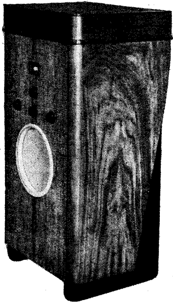
In the Murphy A30 radio-gramophone cabinet the sides are tapered to give a cavity shape which is not prone to any single resonance.
