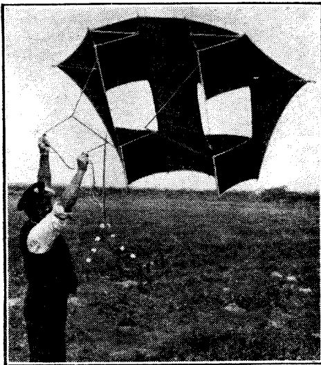
A kite used to fly a half-wave aerial to a height of 325 feet. This is in addition to the trials with 72ft. masts.
