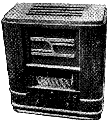
Front view of the Lemouzy receiver showing the additional speaker fret on top.
