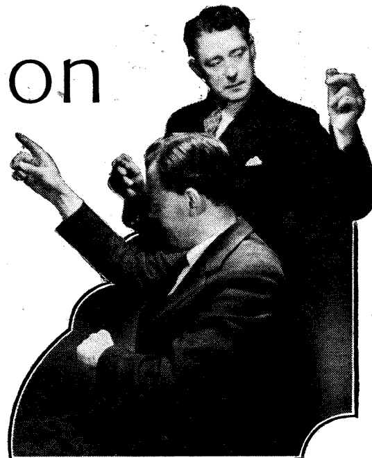
Fig. 2.—A simple experiment demonstrating the loss of sense of direction for sounds originating in the vertical centre plane between the ears.
