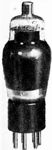
6A7 Pentagrid with a heater rated at 6.3 volts 0.3 ampere.
