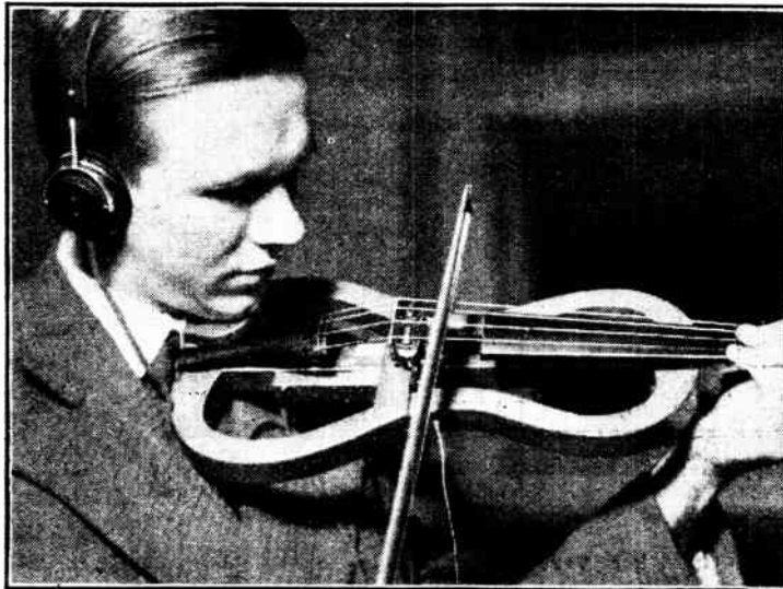
A THOUGHT FOR NEIGHBOURS? Violin practice which only the executant can hear is made possible with the Vierling electric violin, which can be played through a valve amplifier and headphones. Two magnetic pick-ups are used for the strings and another for harmonics. This instrument may shortly participate in an all-Europe electric music broadcast.
