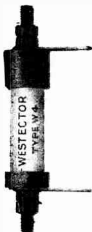
Type W.4. Half-wave Westector. Suitable for use as a radio-frequency or intermediate-frequency detector.
