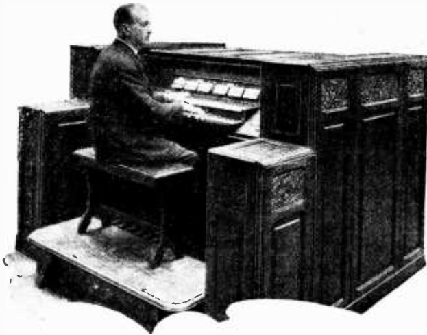
A "RADIO" ORGAN. Poste Parisien broadcasting station is installing a thermionic valve-operated organ of the Givellet-Couplex type. The instrument in the photograph is in regular use at a church in Villemomble, near Paris.
