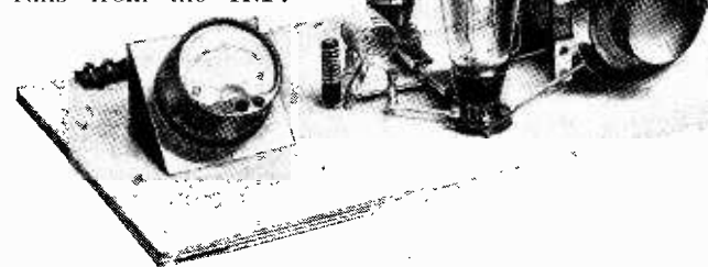
The transmitter, which employs a push-pull arrangement with LS5 valves. These have shown no sign of distress when run for eight hours continuously.
