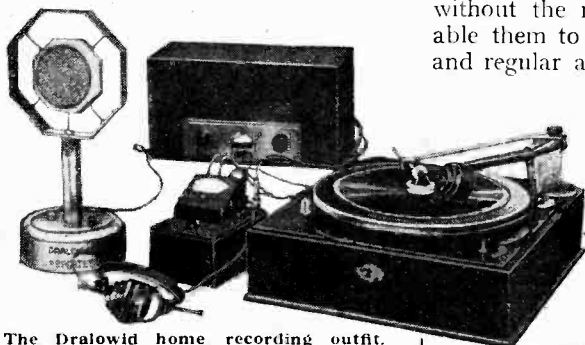
The Dralowid home recording outfit. Records are sent to the manufacturers for baking to render them hard and durable.
