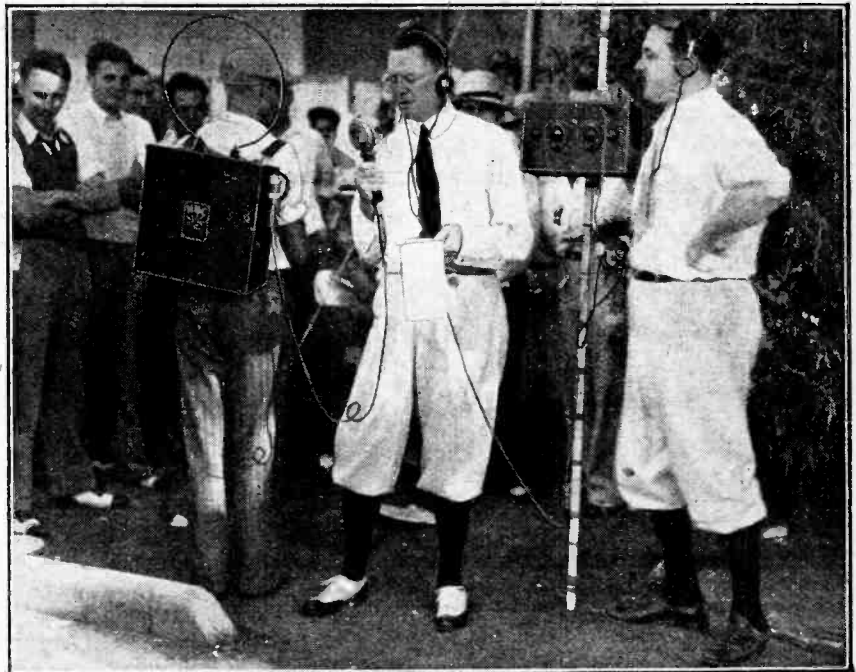
5-METRE TRANSMISSION IN U.S. "Outside broadcasting" in America involves a good deal of pure wireless work before the commentator's remarks reach the landlines. Our picture shows the National Broadcasting Company's new 5-metre transmitting and receiving equipment as used for the first time recently in reporting the American Open Golf Championship.
