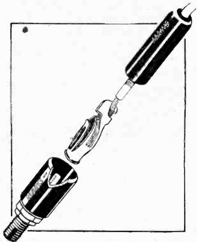
An ingeniously simple shrouded plug and socket (Gripso).
