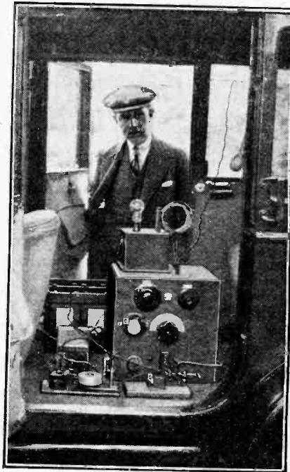
A ROAMING TRANSMITTER. Mr. Maurice Child photographed with the eight-watt transmitter which was tracked by D.F. groups at the recent field day of the Golders Green Society. A loosely coupled Hartley circuit was used and high-tension was obtained from an M-L converter fed by the car accumulator.
