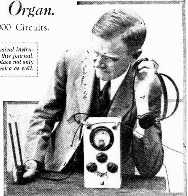
While it was not possible to obtain photographs of the interior of this new apparatus, this illustration reveals that fundamentally the equipment consists of tuning forks used in conjunction with tuned circuits. Actually twelve forks are employed.
