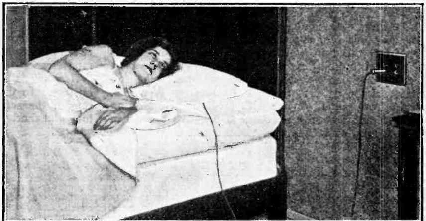
THE WIRELESS PILLOW. Although the idea of concealing a radio reproducer in a pillow is not new it is interesting to note that the device has reached the stage of commercial production. The pillow shown in the picture is composed largely of sponge rubber and is made specially for use in Pullman cars, ships and hospitals.
