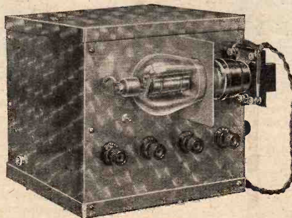
The unit viewed from the back. Note the method of mounting the valve.
