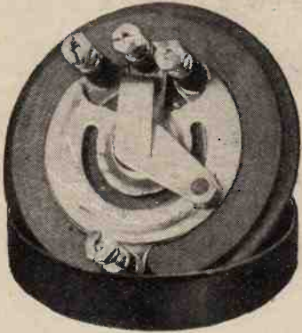
A rocking disc, actuated by a rotating arm, minimises wear on the resistance element in the "Magnum" dissolver.
