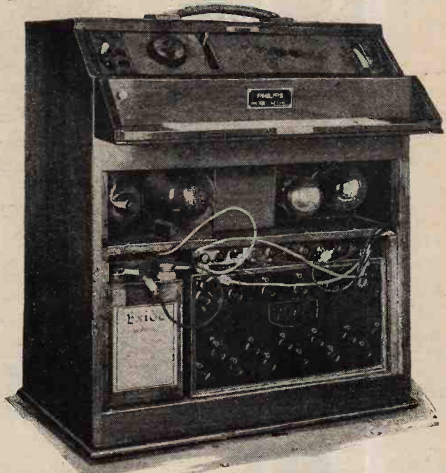
General view of the Philips portable with front panel removed. The layout makes the best use of the space available and gives good accessibility to valves and batteries.
