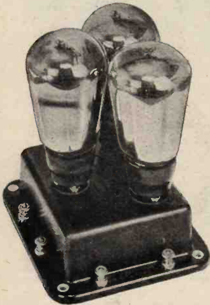
The "C.A.C." low-frequency amplifier which incorporates a combination of resistance and transformer coupling.
