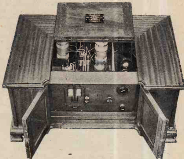
Gambrell 4-valve all-mains D.C. set. Two pentodes are used in parallel as the output stage.
