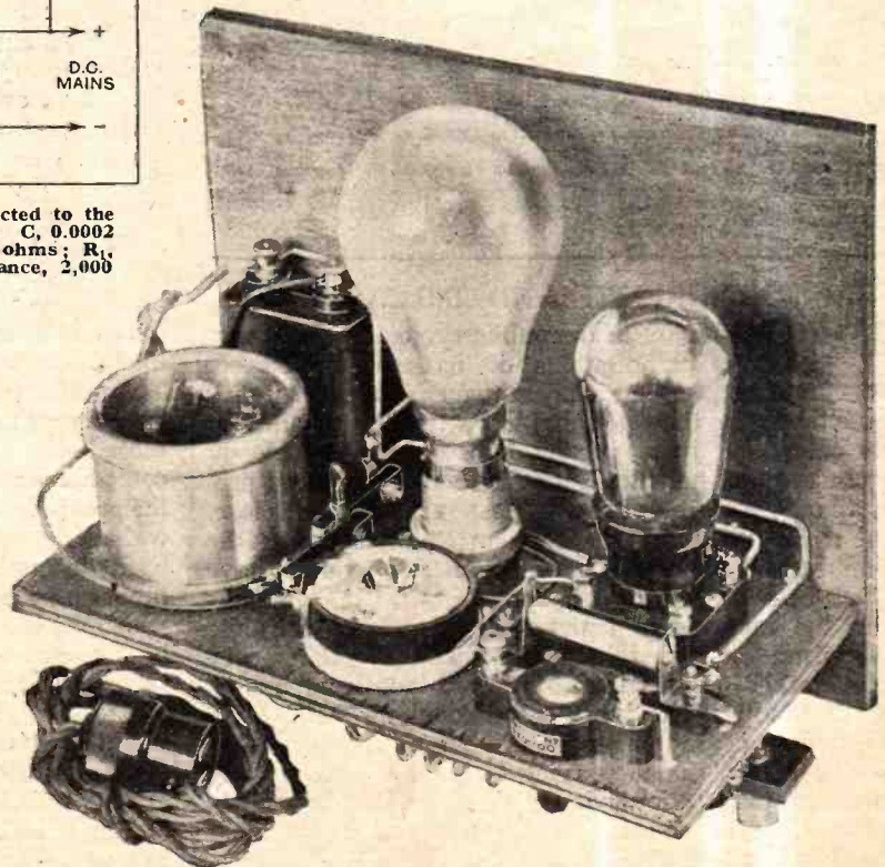
The complete unit. The anode feed resistances are clamped together, and secured to one of the variable resistance terminals.
