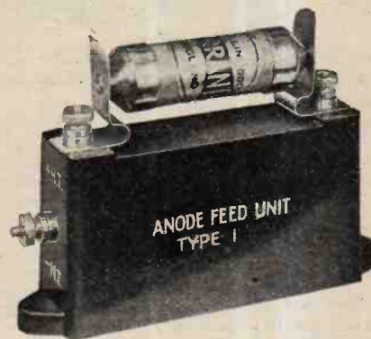
Ferranti anode feed unit consisting of a bypass condenser and decoupling resistance.
