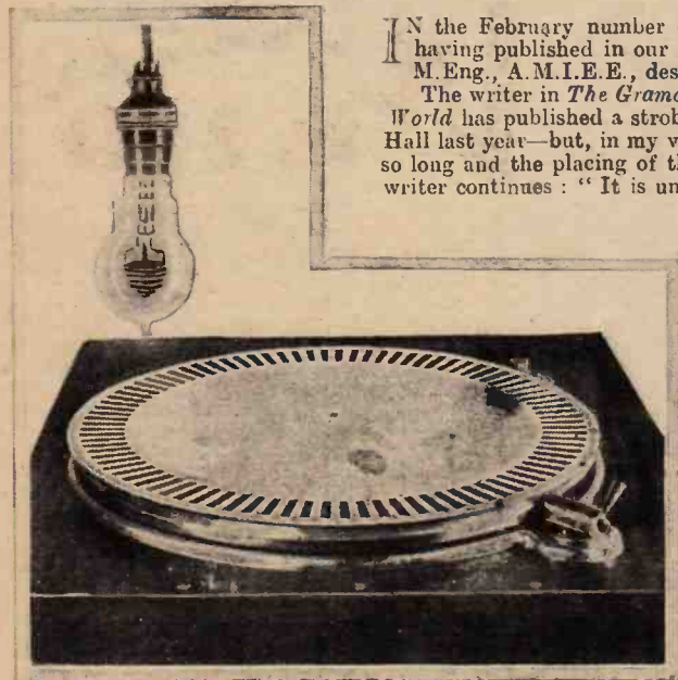
The Stroboscope. Where the electric supply is alternating, a neon lamp can be used to check gramophone turntable speed. With a careful adjustment of the speed regulator the disc will appear to be stationary when illuminated by a neon lamp connected to alternating-current mains.
