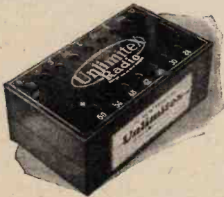
"Unlimitex" 60-volt dry cell H.T. battery. Tappings are provided in 1½-volt steps up to 12 volts and thence in 6-volt steps.
