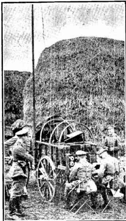
GERMAN FIELD WIRELESS. A photograph taken during the recent Autumn Manœuvres of the German Army. The portable mast is about 20ft. in height.
