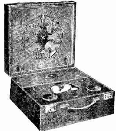
The Lissen portable to be found on Stands 184 to 186. A 5-valve receiver with one dial tuning.
