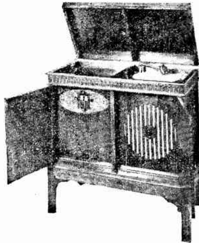
Gambrell's version of an all-electric radio gramophone. Four valves are used, including a screen grid and a pentode. Shown on Stand 62.
