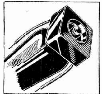
Economical of weight and space: Amplion method of mounting "aperiodic" H.F. transformer on the anode terminal of an S.G. valve.
