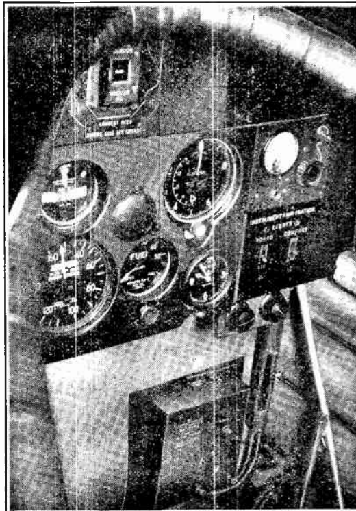
THE RADIO BEACON INDICATOR is the topmost instrument seen in this view of the cockpit. The two white spots mark the extremities of reeds which vibrate vertically when the radio beacon is tuned in.
