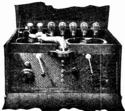
Barraclough's heavy duty gramophone amplifier. Note the two turntables.
