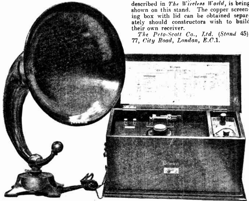
Valve crystal receiver with valveless amplifier.
