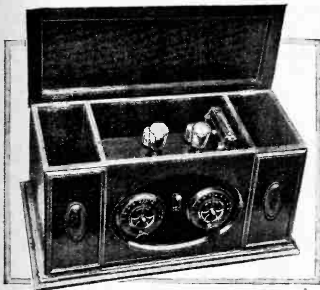
Accessibility of interchangeable components is a noteworthy feature of the Terry Two-valve set. Note separate compartments for H.T. and L.T. batteries.
