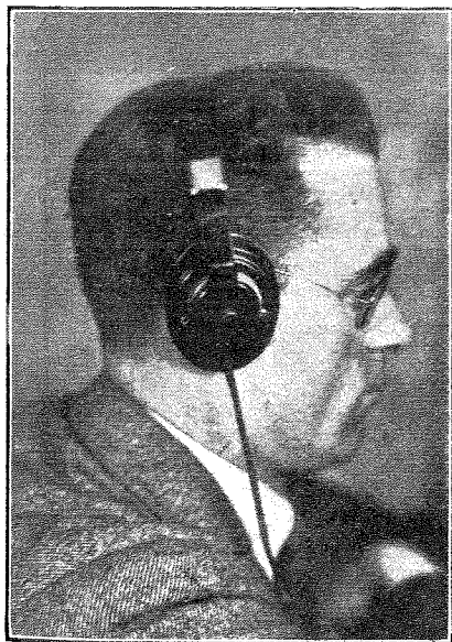
Attachment to the head is obtained by the ear cap instead of the clamping action of the headband.
