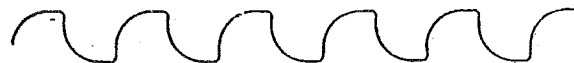
Fig. 4.—Current wave-form of modulation in transmitting aerial—slightly exaggerated to show the effect of electromagnetic inertia.
