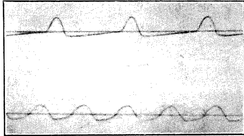
Fig. 6. Oscillograph records showing the waveform of the oscillations set up by a zincite detector.
