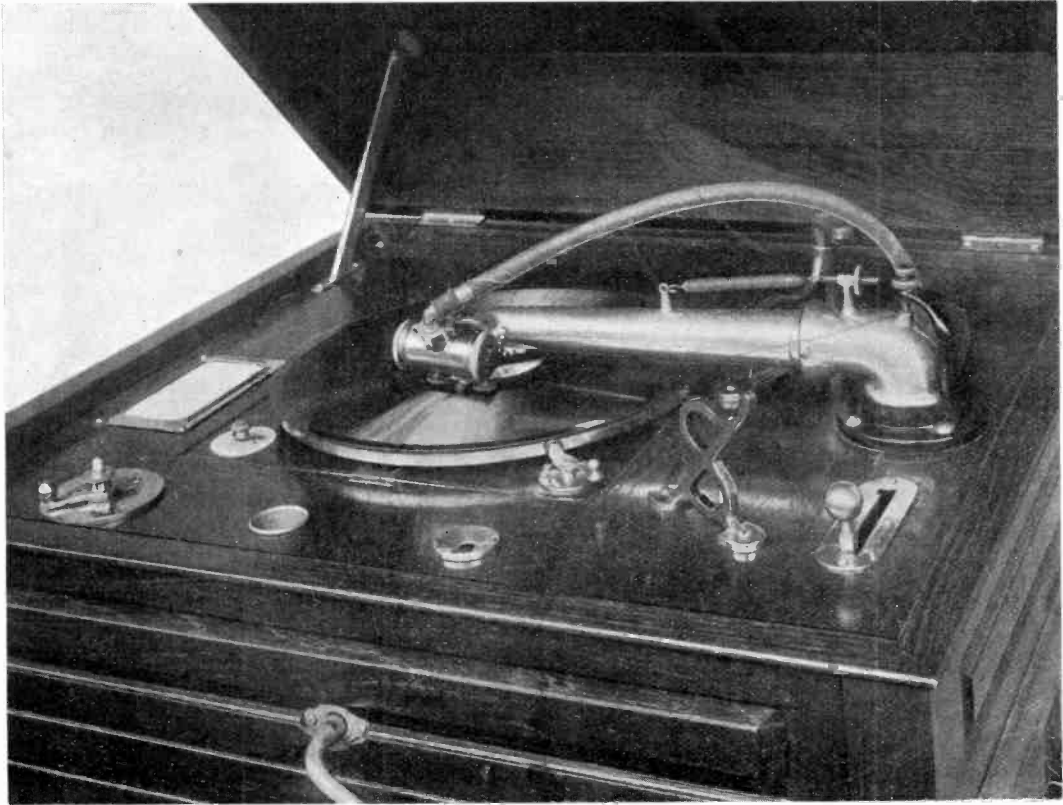
Fig. 32. The tone arm, valve, air delivery pipe, and Record on a Creed Stentorphone.
