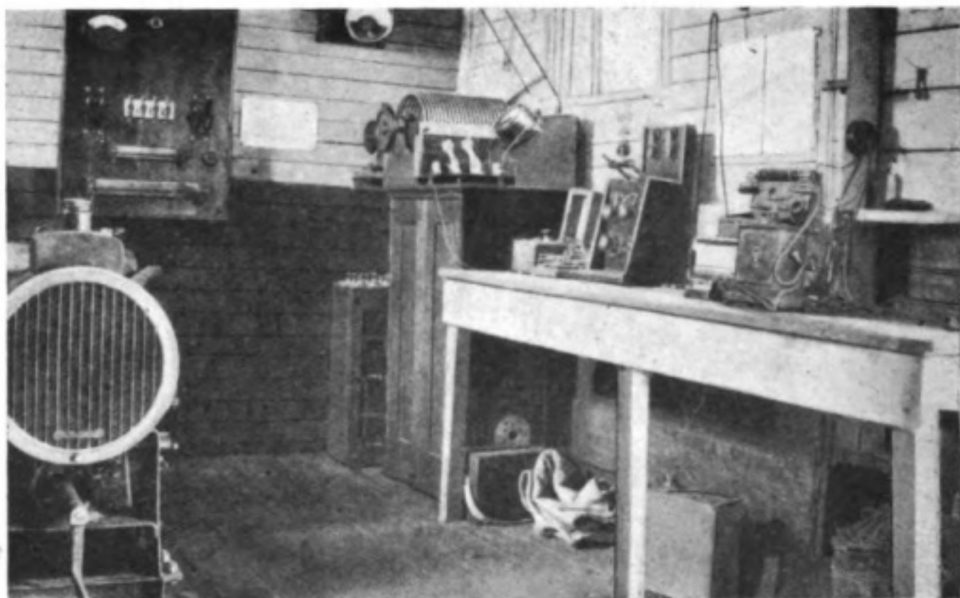
Kem Wireless Station, showing 3-k.w. spark set. This station is also fitted with a 250-watt C.W. valve set.
