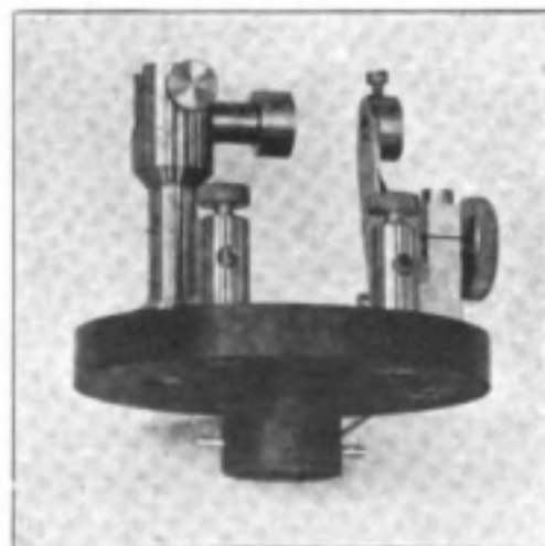
FIG. 5. ANOTHER FORM OF THE HOLDER SHOWN IN FIGURE 3. THIS IS MADE INTERCHANGEABLE WITH THE FLEMING VALVE
