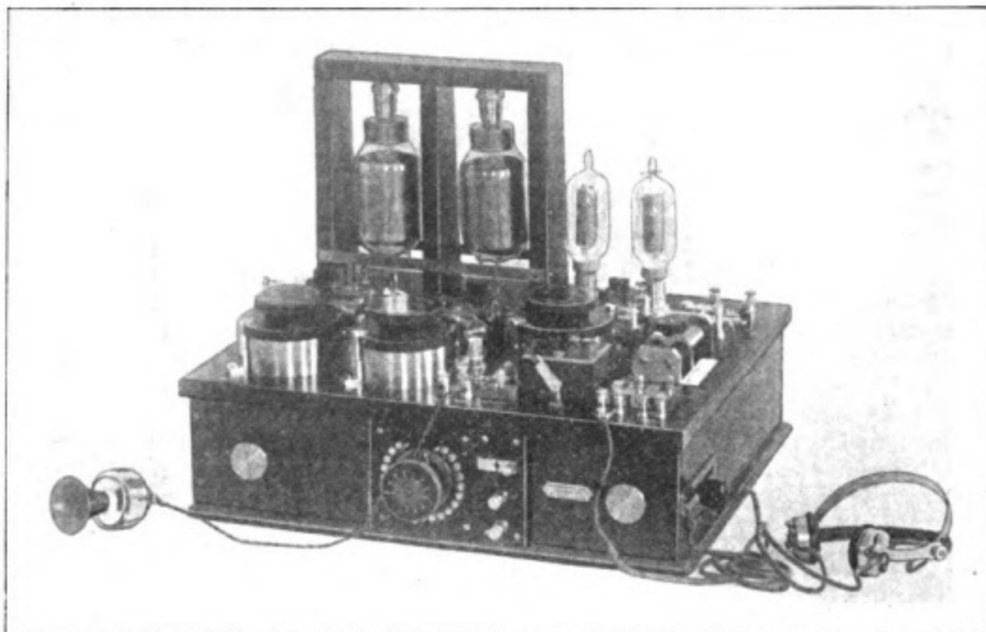
Marconi Short Distance Wireless Telephone, showing Combined Transmitter and Receiver, and Telephone Receiver.
