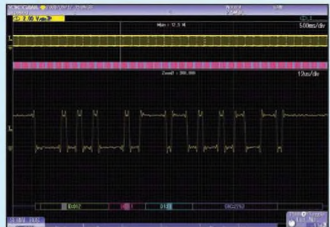
CAN waveform of 12.5 M points (5 sec duration) showing use of the zoom window
