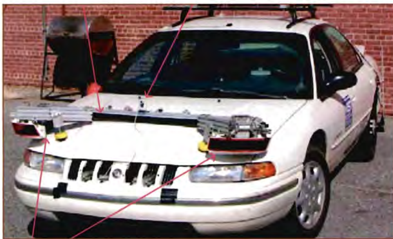
Test-bed vehicle with dual-head laser range scanner
