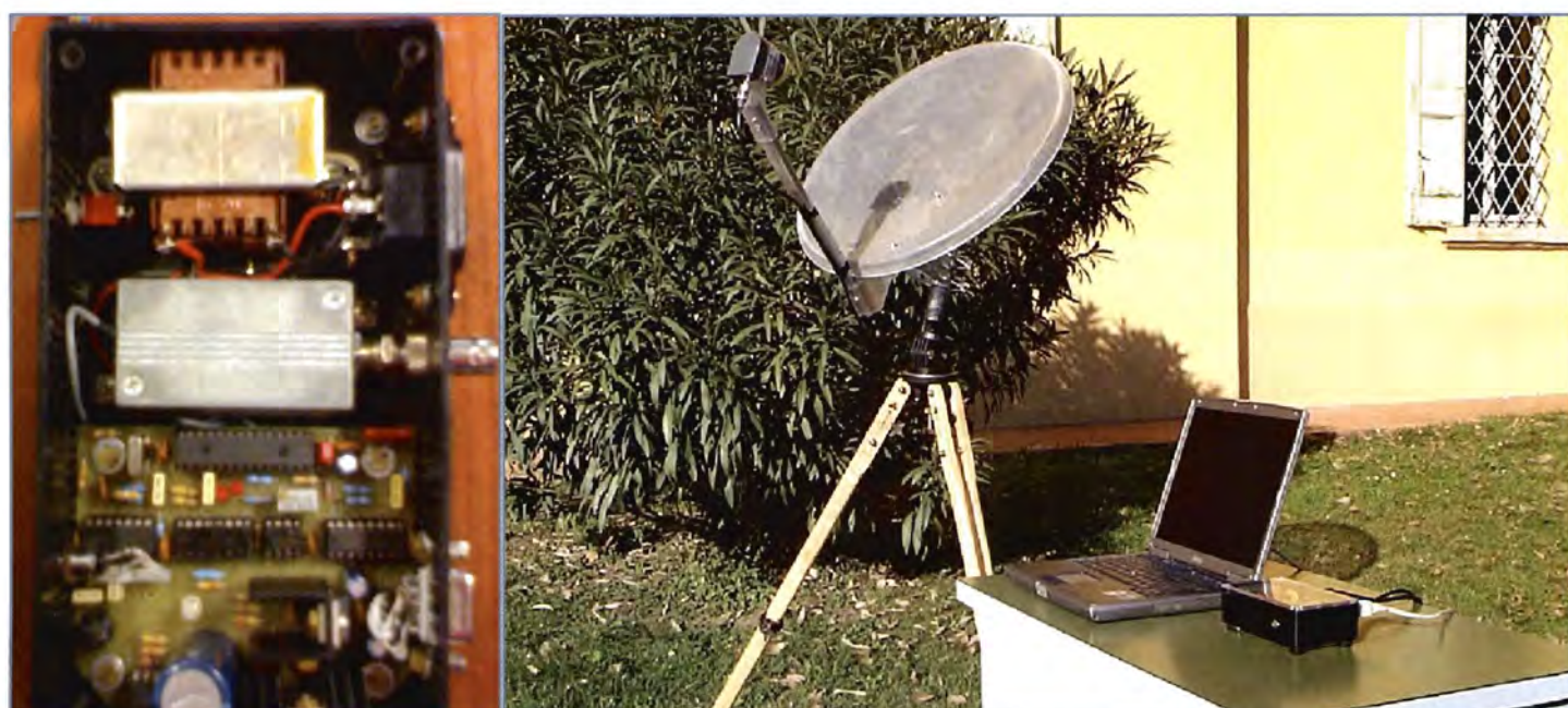
Figure 12: The implemented receiver (left), the teaching radio telescope operating at Villa Griffone (right)
