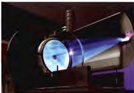
This Cymer EUVL source is a laser produced plasma generated by carbon dioxide laser radiation onto a tin droplet target
