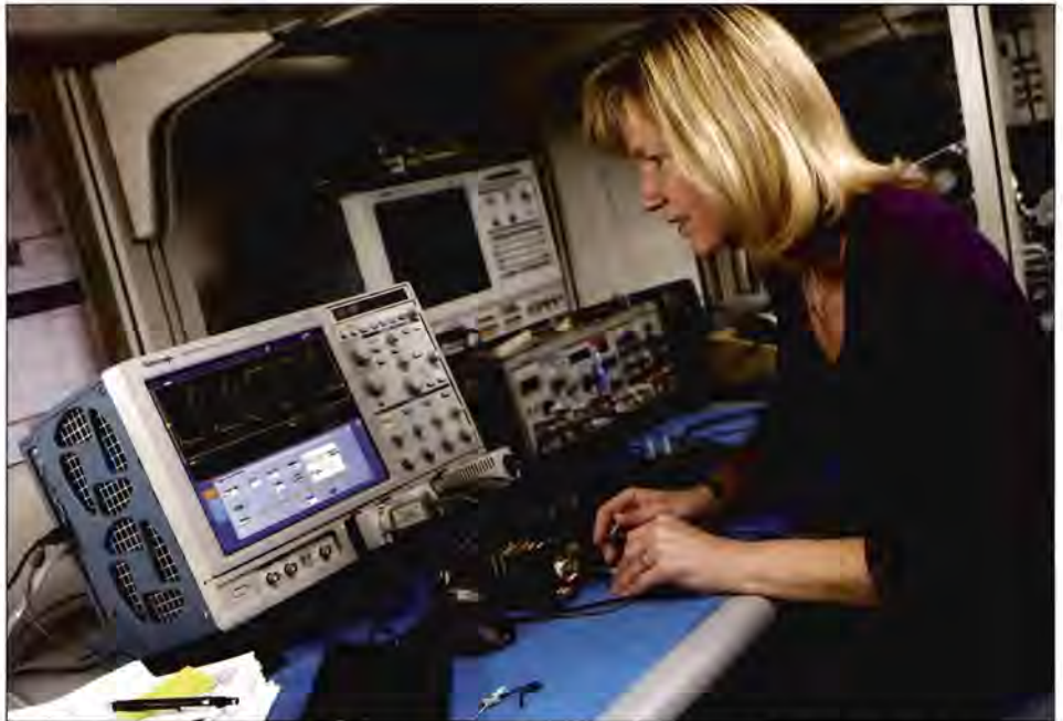
Figure 1: The Tektronix DPOPWR power measurement and analysis software runs on the company's DPO7000 series of Digital Phosphor Oscilloscopes (DPOs)
