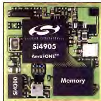
It doesn't get smaller than this – Silicon Laboratories's AeroFone Si4905 in a 12x12mm BGA package
