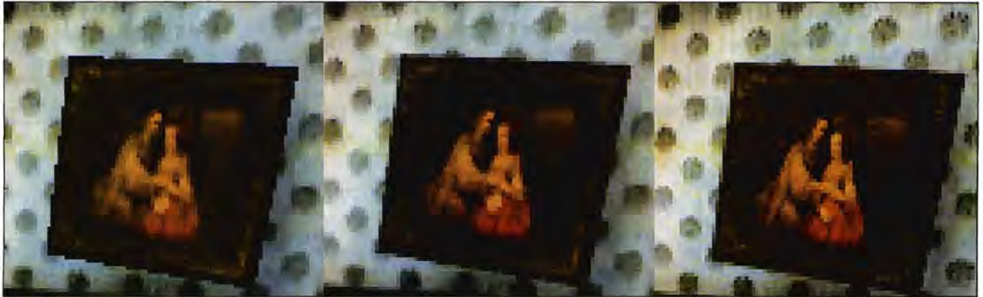
Figure 1: The improved visual quality produced by 4x and 16x FSAA. Note the significant reduction in jaggies surrounding the frame between no FSAA and 4x FSAA, and the additional detail in the wallpaper and painting with 16x FSAA.
