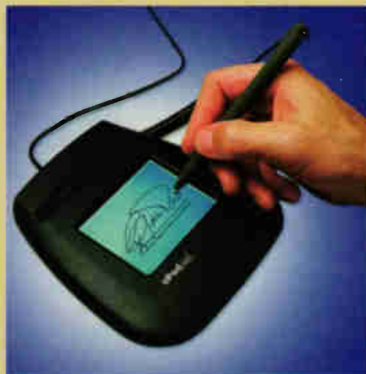
An LCD and touchscreen have been combined by Interlink Technologies to create a system for capturing digital signatures. The ePad-ink can add a signature to documents in standard software packages such as Microsoft Word, Access, Outlook and Adobe Acrobat. The LCD allows the document being signed to be displayed as they sign. The ePad-ink can also capture handwriting biometrics, including stylus pressure and timing.
