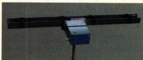
Fig. 6. Ferrite Aerial and Amplified Short Dipole tuned at 138.83kHz and used in the Tests.
