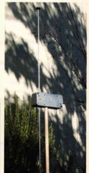
Fig. 6. Ferrite Aerial and Amplified Short Dipole tuned at 138.83kHz and used in the Tests.
