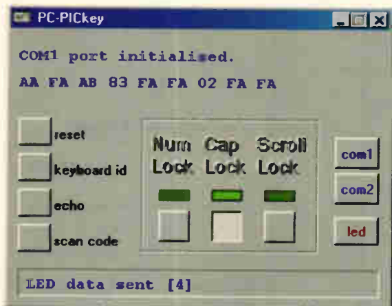
Fig. 14. Windows PC screen showing various command options and response received from the keyboard.
