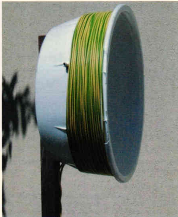
Fig.11. The Loop 18, an 18 turn, 31 cm diameter reference loop.
