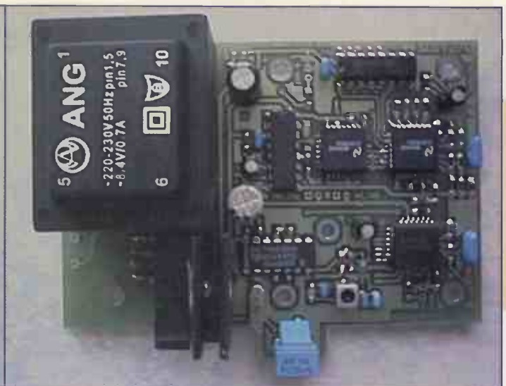
Fig. 12. A second view of the internals of the SDIT270. The mains power supply is integrated into the unit, but you can easily adapt the design to use an external wall-mounted adapter.
