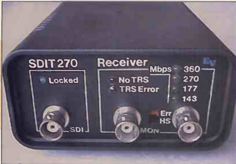
Fig. 9. Front View of the SDIT270 SDI generator and receiver. The device is housed in a plastic copper-shielded box.
