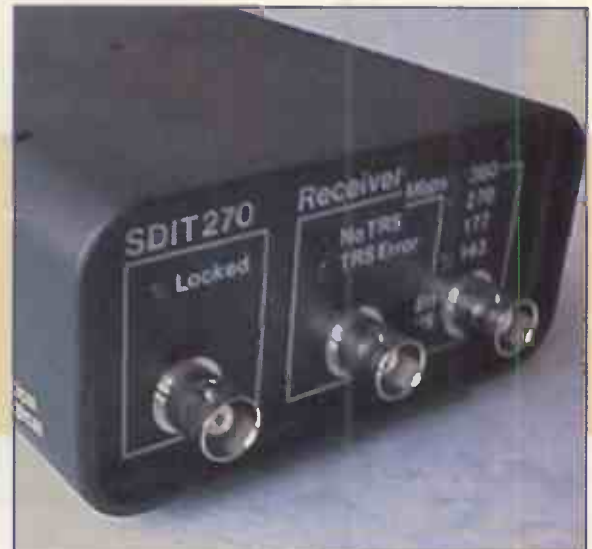
Fig. 10. General view of the SDIT270 device. The position switch, which controls the output test pattern, is on the device's side panel.
