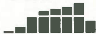
Fig. 5. Each press of the scan button updates the spectrum bar graph and displays the next frequency up the scale, represented by the left-most digit, together with its amplitude, which in this case is 178mV.
