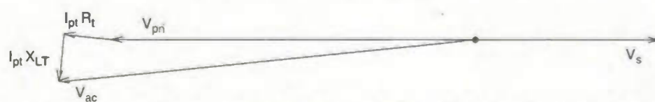
Fig. 5. Showing the corresponding voltages (secondary resistance and leakage inductance referred to the primary). X_{LT} is the total leakage reactance at the supply frequency, referred to the primary.
