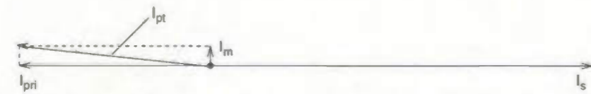
Fig. 4. Showing the currents flowing, assuming N=2 , I_m = I_{pri}/10 . Although the primary and secondary currents are different, their ampere-turns product on the core cancel exactly.
