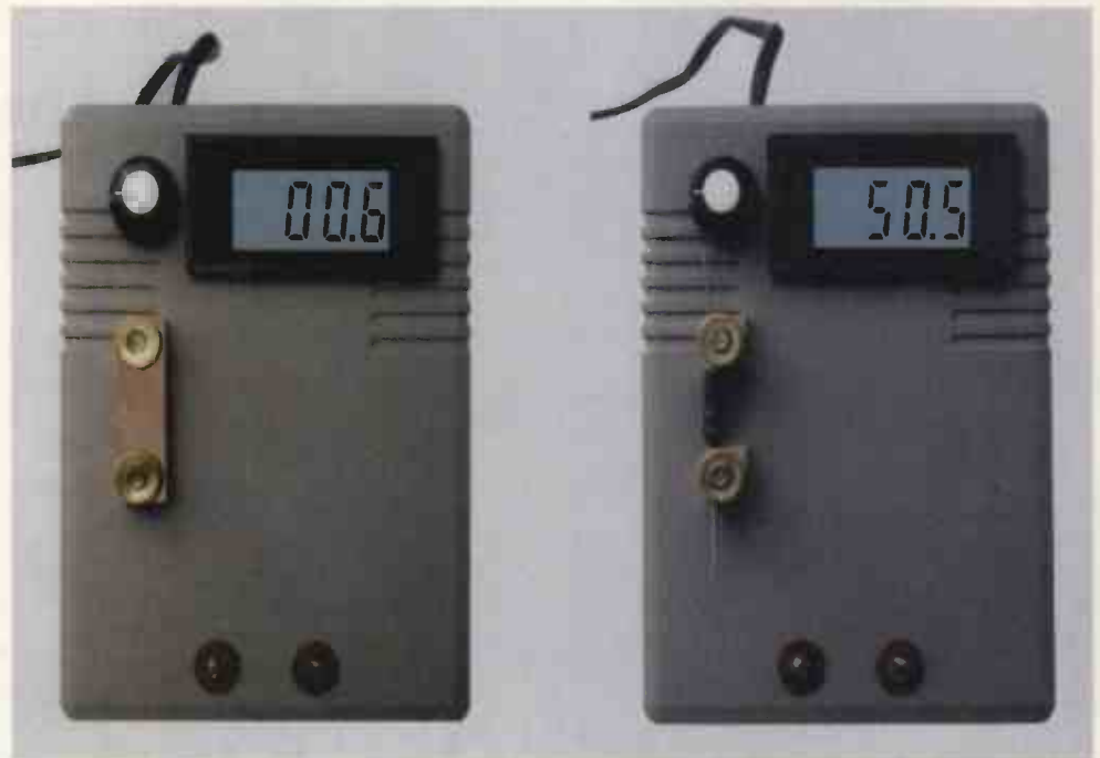
On the left is the milli-ohm meter with the copper shunt showing a reading of 0.6m \Omega . Right is a 50m \Omega , \pm 1% resistor being measured. Subtract the 0.6m \Omega residual and the reading becomes 49.9m \Omega .
