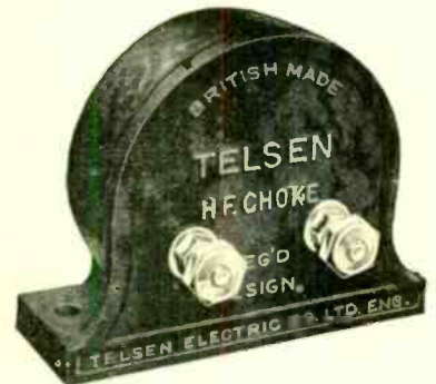
Telsen H.F. Chokes , designed to cover the whole waveband range from 18 to 1,000 metres, extremely low self-capacity, shrouded in Genuine Bakelite. Inductance 150,000 microhenries, resistance 400 ohms. Price 2/6 each
