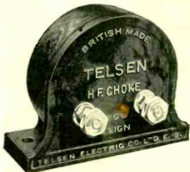
Telsen H.F. Chokes designed to cover the whole wave-band range from 18 to 4,000 metres, extremely low self-capacity. Inductance 150,000 microhenries; resistance 400 ohms. Price 2/6 each.
