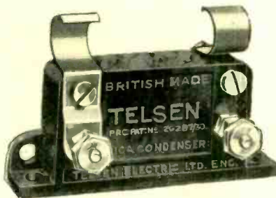
Telsen (Mica) Condensers made in capacities up to .001 mfd. Prov. Pat. No. 20287/30, supplied complete with Patent Grid Leak Clips to facilitate series or parallel connection; can be mounted upright or flat, tested on 500 volts. Genuine Bakelite Mouldings. Price 1/- each
