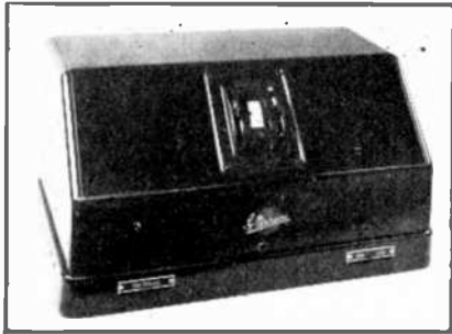
The Marconiphone Model 47, all-mains A.C. receiver—the only metal-cased set in the range.
