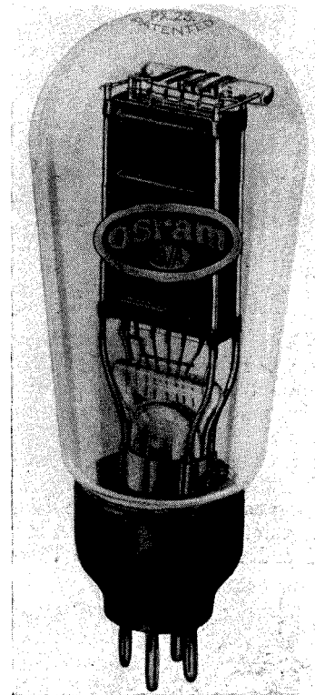
(Above) This photograph of an Osram PX25—a big triode output valve—shows clearly the rectangular plate. Above this one can see the beginning of the grid, and the filament which is suspended vertically. This is typical of modern three-electrode valve practice.
