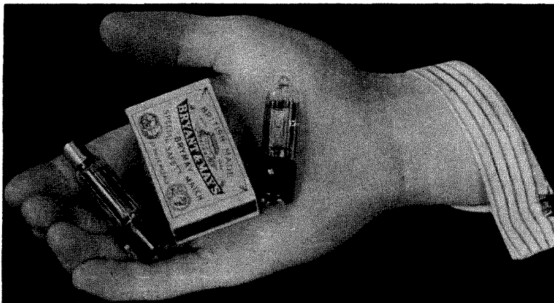
Just how small the new midget valves introduced by Hivac really are can be seen from this photograph. Although physically small, their electrical characteristics approximate to the standard of the full-size valves
