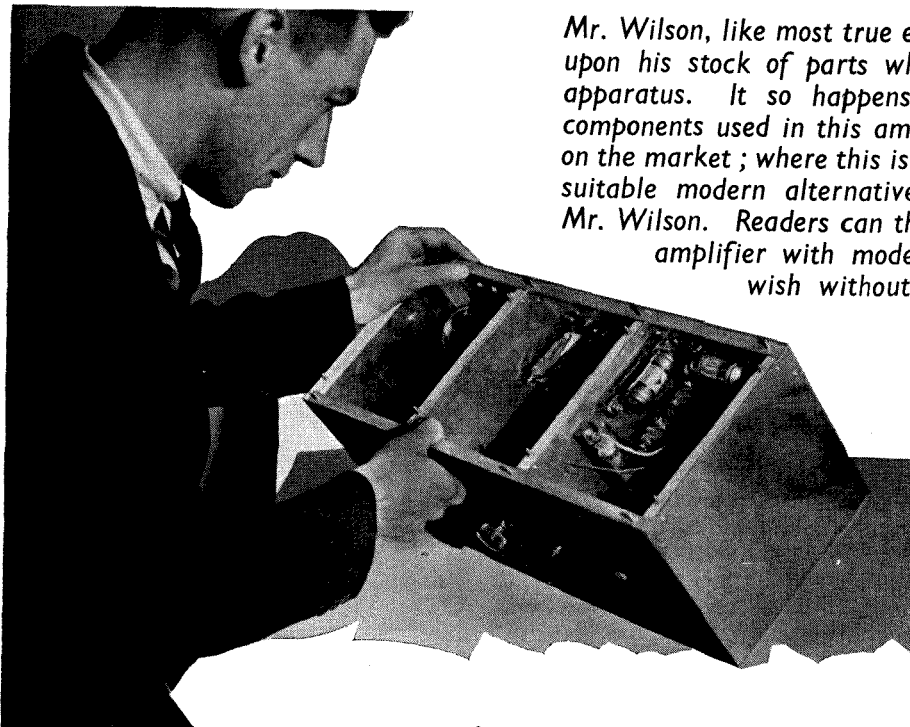
The amplifier built by P. Wilson is arranged in three distinct parts in one metal box. The power pack is constructed as a separate unit
