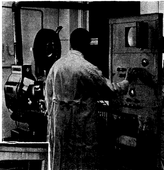
Inside Berlin's television transmitter showing the film-scanning apparatus with a cathode-ray check tube. An arc light consuming 250 amperes is used for the 180-line scanning
