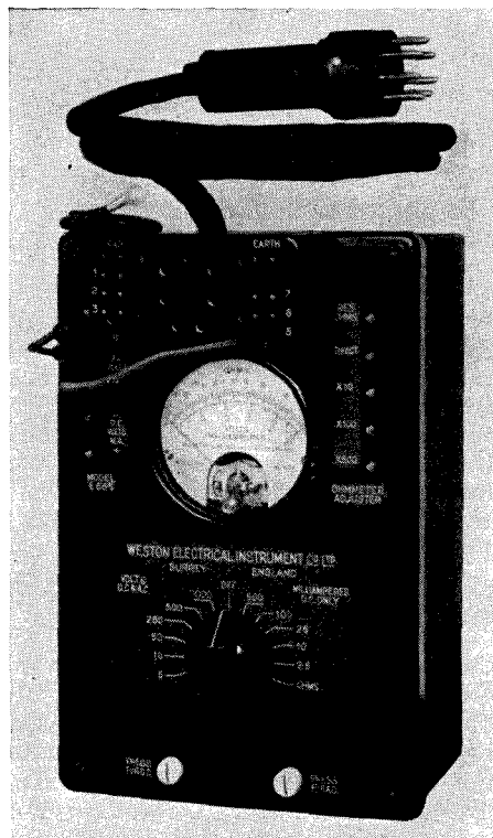
The Weston Analyzer is a combination test instrument of great value in service work. It covers a great variety of voltage, resistance and current measurements
