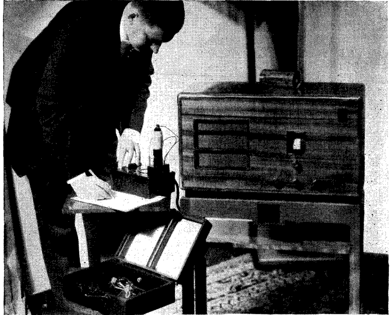
Much time and trouble in set servicing can be saved if suitable and good test apparatus is used. Here you see a service engineer with the Weston Analyzer in use
