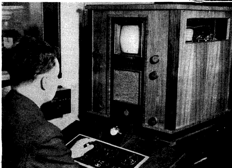
Whilst sound and vision are being transmitted an engineer sits in front of a check receiver making sure that all adjustments are right. Note the curved end of the cathode-ray tube
