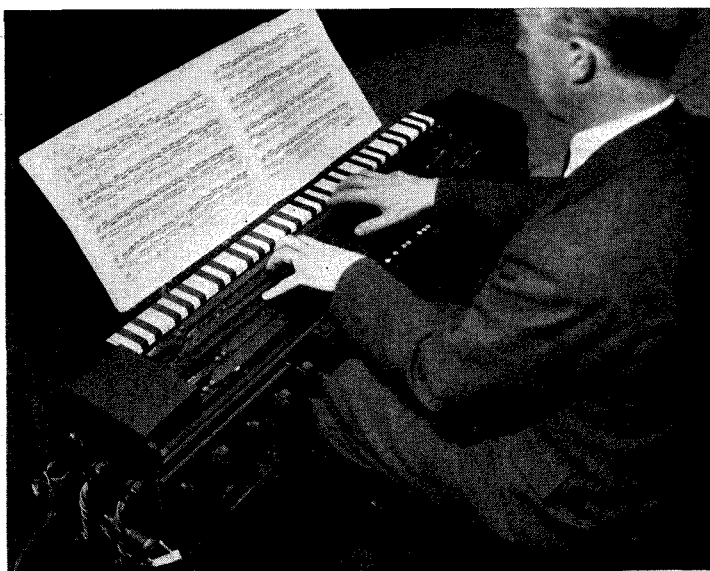
A close-up view of the Hellertion. Five keyboards (shown absolutely plain without any markings) are seen below a strip of wood coloured to resemble the keys of an ordinary piano. This dummy keyboard acts purely as a guide for the beginner at the instrument
