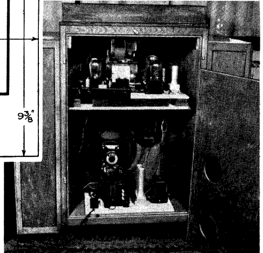
Everything fits into place with ample room to spare. The back of the cabinet is provided with sound outlets to prevent box resonance effects
