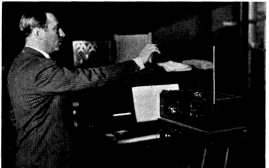
Showing Professor Theremin's ether-wave piano. It is controlled by the backward and forward movement of a hand (in thin air) in front of a small rod protruding above the instrument. The instrument has been demonstrated many times in this country; many will remember a broadcast given by a leading exponent
