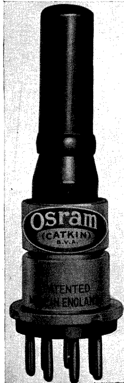
An unusual valve, the Osram Catkin has an anode which also takes the place of the glass bulb of the ordinary valve. This form of construction ensures exceptional rigidity and robustness
