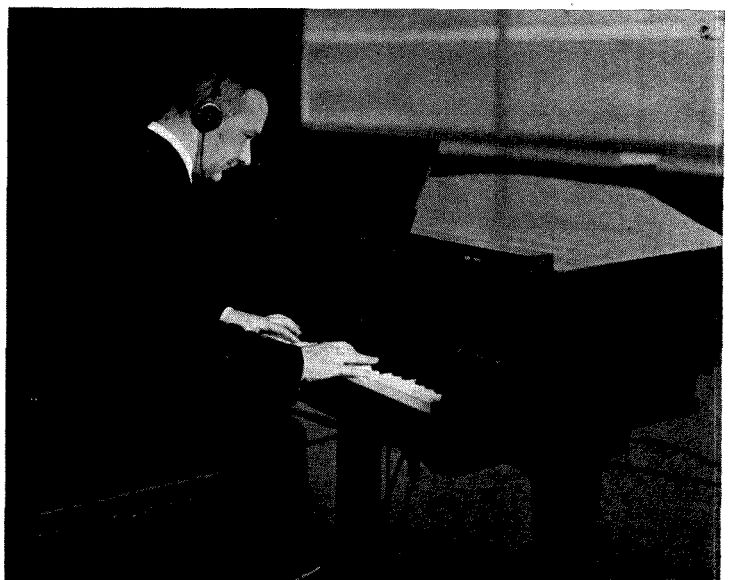
The loudspeaker on the Neo-Bechstein piano can be disconnected and a pair of headphones substituted. A boon to the household when the children are at practice!
