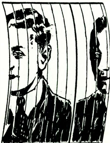
If you should have a picture split vertically, as shown by the drawing, allow the motor to revolve a little faster and you will find that as the picture slowly travels up it will also move sideways until the picture is completely in view.
