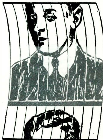
If the picture is split horizontally a very slight alteration of speed will correctly frame the image
