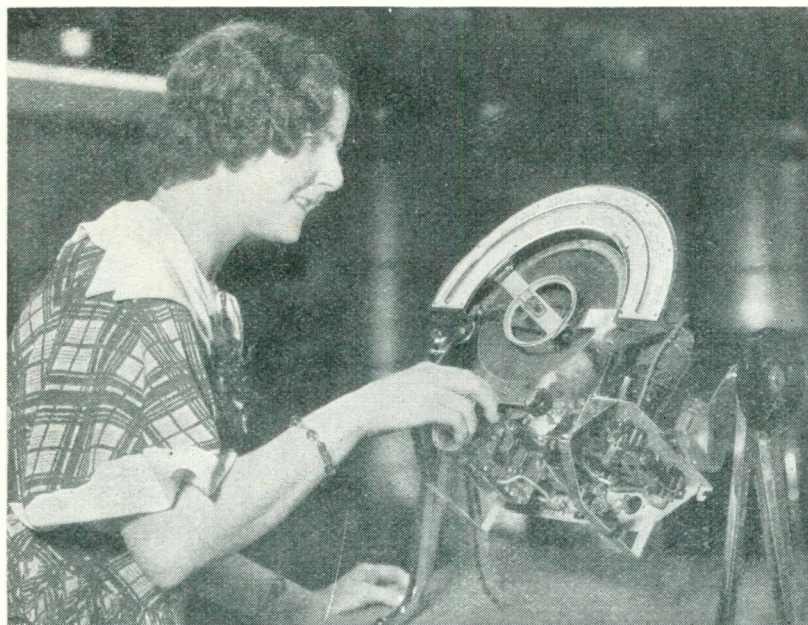
SHOWING MODERN COMMERCIAL SET CONSTRUCTION Showing the chassis of the Ekco model 65—the set in the circular bakelite cabinet. Tone control is embodied in this really ultra-modern design. Note the unusual position of the three-gang condenser
