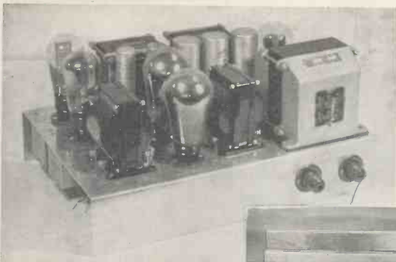
(Above) A view of the completed amplifier and mains section. The fuses are incorporated in the mains transformer. The two low-frequency valves are seen on the extreme left and the output triodes between the two transformers
