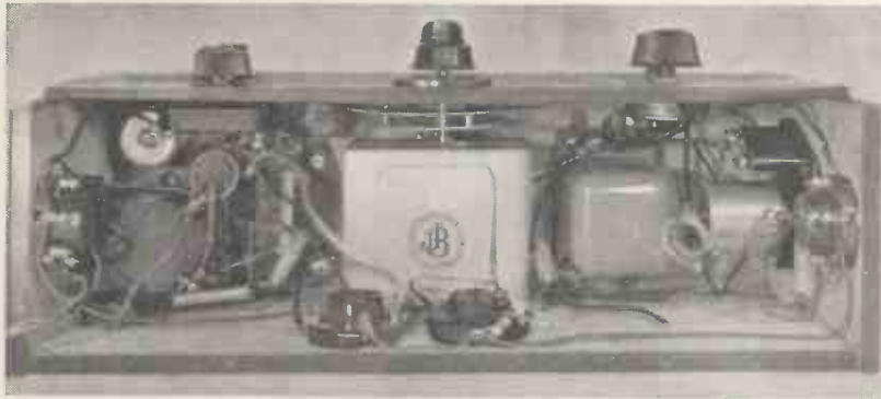
WITH THE SCREEN REMOVED This view shows clearly the layout of the Tyers Portable. If the construction is attempted as shown by the drawing on page 14, there should be no difficulty whatsoever. A metallised-wood screen fits between the valve holders and the rest of the set
