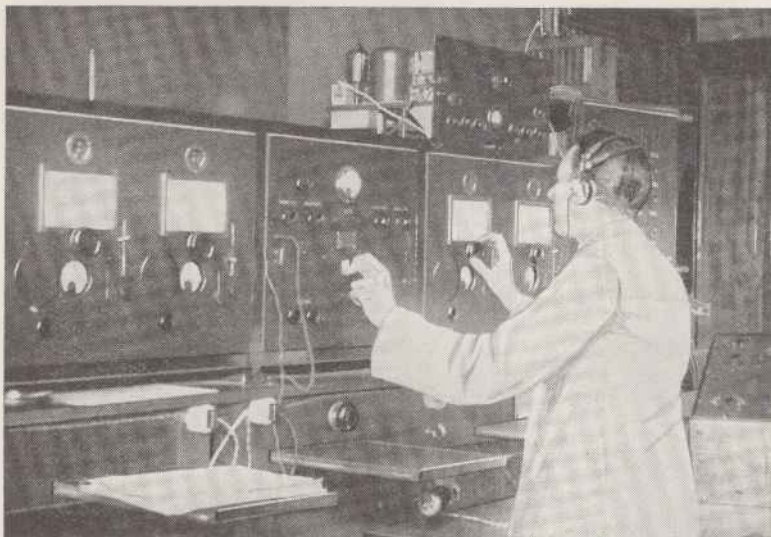
CENTRE OF THE I.B.U.'S TECHNICAL WORK Some of the apparatus used at the now famous Brussels Checking Station where the wavelengths of all European stations are checked for accuracy
