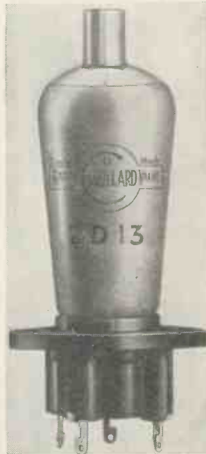
Two good examples of double diodes. (Left) The Ostar-Ganz with a 200-volt heater and (right) the Mullard with a 13-volt heater
