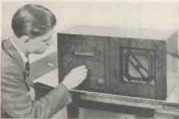
"This new set is in a horizontal walnut cabinet. . . . The receiver is on the left-hand side with the loud-speaker behind an attractive grille on the right"
