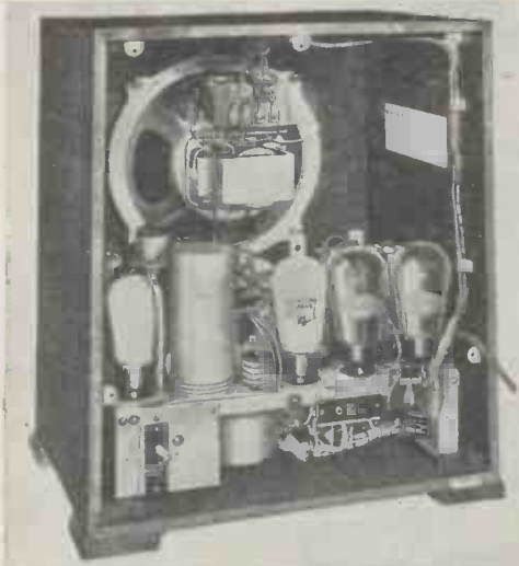
"There is no need to say much about the circuit. There are four receiving valves and a full-wave rectifier"
