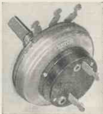
The Ferranti combined potentiometer and switch is quite shallow and has soldering lugs
