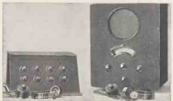
A boon to the deaf. The Multitone deaf-aid set with a distributing panel for use in schools and institutions
