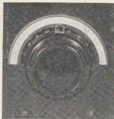
SUITABLE VERNIER DIAL This Burndept Eshovernier dial is particularly suitable for incorporation in this tester. Calibrations can be marked on the paper scale provided
