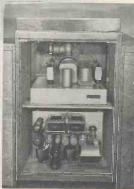
(Above) A view of the completed amplifier and mains section. The fuses are incorporated in the mains transformer. The two low-frequency valves are seen on the extreme left and the output triodes between the two transformers
