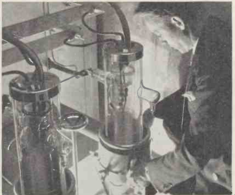
PUTTING A 100-KILOWATT VALVE IN ITS HOLDER!
