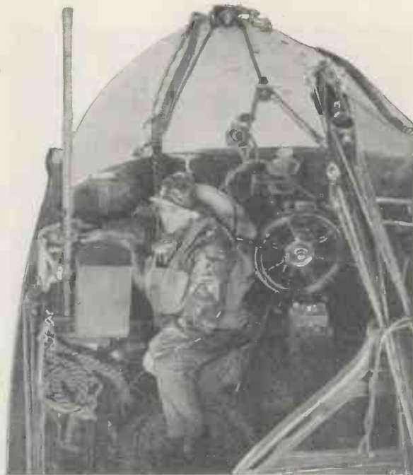
Hythe lifeboat has been permanently fitted with a wireless set specially designed for use in an open boat by G. S. Woodman. To stand up to the elements of the sea, the set has been built into a watertight metal container
