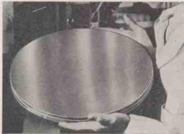
Columbia photo "BLANK" FOR A COMMERCIAL RECORD Note the glass-like surface of this wax blank, ready for recording. Most home-recording outfits use aluminium blanks
